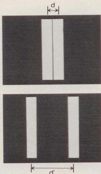
**Fig 11.** Results of an experiment performed with a photo slit lamp (Nikon FS-2). *Top* was obtained on a cover glass 0.17 mm thick with a set-up according to Figure 10 *left*. By intercalating a contact glass of magnifying power  $\times 2$  according to Figure 10 *center*, *bottom* was obtained. The slit width and the angle between illumination beam and microscope were the same for both pictures. Image separation  $d' = 4d$ .
