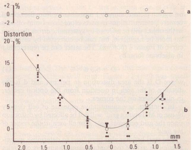
**Fig 8.** Apparent relative area distortion (%) of small circles on a spherical surface of 7.75 mm radius photographed with the Nikon FS-2 photo slit lamp, *a*, directly, and *b*, with intercalation of the contact glass. Abscissa is distance of circle centers from the vertex of the sphere. Full points are values of individual circles; hollow points are their mean values at a given eccentricity. The latter are approximated by curve D (see eq. [1]) when the contact glass is used.
