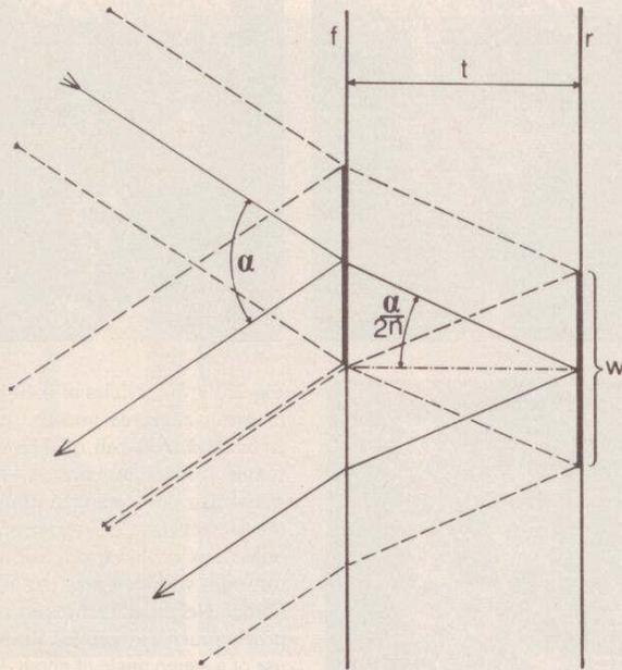
Fig 9. Course of rays at a membrane observed with the slit lamp. The drawing corresponds to a horizontal cross section of Figure 10 left;  $f$  and  $r$  are the front and rear surfaces of a transparent membrane of thickness  $t$  and refraction index  $n$ , on which two images of the slit are formed;  $w$  is their width and  $\alpha$  is the angle between slit beam and microscope axis.
