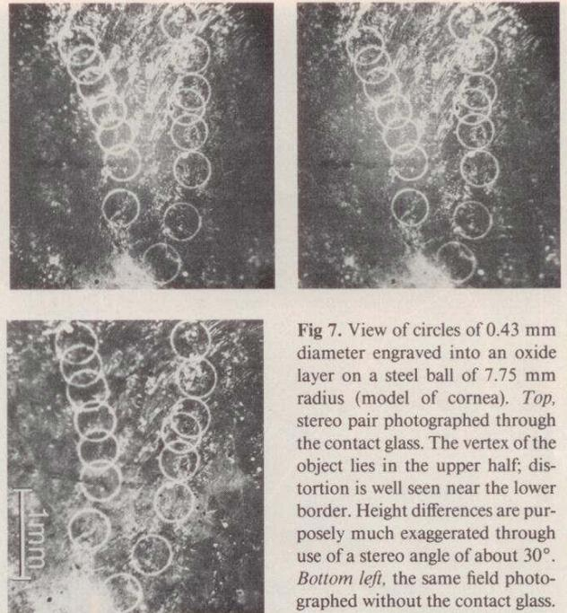
**Fig 7.** View of circles of 0.43 mm diameter engraved into an oxide layer on a steel ball of 7.75 mm radius (model of cornea). *Top*, stereo pair photographed through the contact glass. The vertex of the object lies in the upper half; distortion is well seen near the lower border. Height differences are purposely much exaggerated through use of a stereo angle of about  $30^\circ$ . *Bottom left*, the same field photographed without the contact glass. There is practically no distortion.
